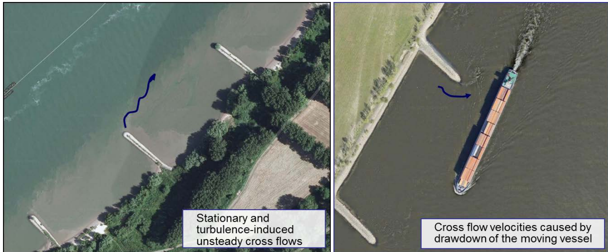
Figure 3: Illustration of turbulence- (left picture) and ship-induced flows (right picture) in the vicinity of groins.
