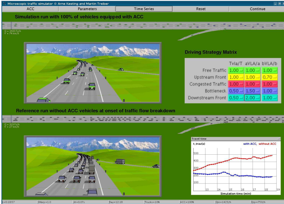
Fig. 2. Screenshot of our traffic simulator, showing the on-ramp scenario studied in Sec. 4.1. In our visualization, the current traffic state of each ACC vehicle is displayed by a changing vehicle color allowing for a direct, visual assessment of the detected states. In contrast, non-ACC vehicles are displayed in grey color. The parameters of the strategy matrix can be changed interactively by the researcher in order to test new strategy matrices directly. For matters of illustration, two simulation runs are displayed. In the upper simulation, 100% of the vehicles are equipped with the ACC-based traffic assistance system. The different vehicle colors indicate the locally detected traffic states. The reference case without ACC equipment (grey vehicle color) displayed in the lower simulation window shows congested traffic at the bottleneck. In both simulations, the same time-dependent upstream boundary conditions have been used (cf. Fig. 3).
