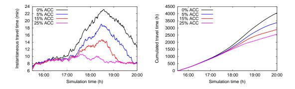
**Figure 3:** The instantaneous and cumulated travel times for different ACC equipment levels. The left diagram demonstrates the strong effect of a traffic breakdown on the resulting travel times, while the cumulated travel time indicates the impact of congestion on the overall system.
