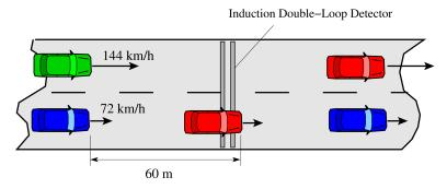
? determine  $Q^{\rm tot}$ , V and  $\rho^{\rm tot}=Q^{\rm tot}/V$  for the total cross-section of two lanes and compare with the "true" density and spatial mean speed
