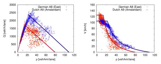
► German A8-East near Munich: Higher maximum speed and lower capacity compared to the Dutch A9 near Amsterdam
