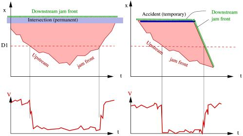
Analysis of a single detector station cannot resolve the upstream-downstream ambiguity when traffic gets free again at the cross-section
