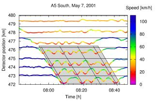
Determine the time shifts  $\tau_{kl}$  for the maxima of the CCF and the individual wave speed estimates  $w_{kl} = \Delta x_{kl}/\tau_{kl}$  with  $\Delta x_{kl} = x_l - x_k$  the distance between the respective detector stations
