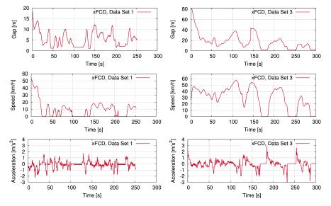
XFC data are normal FC data augmented by additional information provided by vehicle sensors via the internal ehicle data bus (CAN bus)
