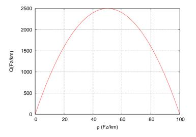
(d) Speed-flow diagram: Repolace in  $V(\rho) = V_0 (1 - \rho/\rho_{\text{max}})$  the density  $\rho = Q/V$  (hydrodynamic relation):
